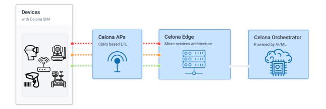
The system consists of the essential functions detailed in Figure 1: System Architecture. The Celona Orchestrator performs AP authentication, validates the AP's serial number, determines the network the AP needs to connect to and finally directs the Celona AP-10 to the serving Celona Edge.
