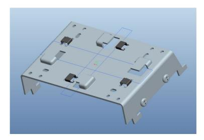
For drop-celing mounting, position the rear clips on the mounting bracked to the ceiling grid and twist counter-clockwise until the springs lock into place. Two sets of rear clips on the mounting bracket support both 24mm and 15mm T-grid rails.
