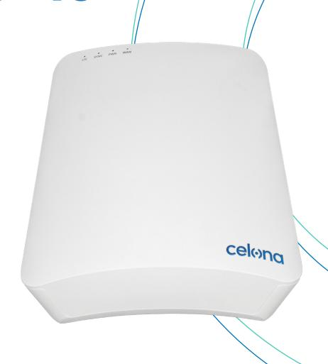
The Celona AP-10 can be mounted on indoor ceilings or walls in various indoor environments. They are powered via Power over Ethernet (802.3at PoE+) or via AC power. They take advantage of existing Ethernet/IP infrastructure for network connectivity. After installation these access points auto-discover the Celona Edge and Celona Orchestrator over any enterprise IP network to enable a plug and play deployment model.
