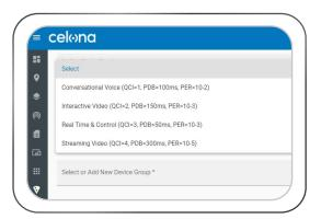
Once a bearer type and QoS class option is selected, the final step is to assign the appropriate Application(s) and custom device group(s) to the MicroSlice.
